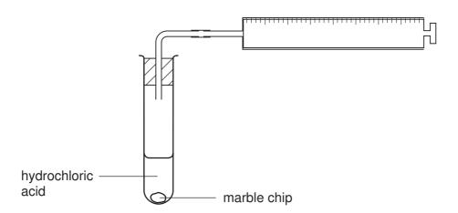
5 test-tubes were put in a rack. To each test-tube was added 10 cm<sup>3</sup> of different solutions of aqueous hydrochloric acid and a marble chip. The marble chips were the same size.
